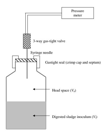
Test vessels in an environment of 35 °C  $\pm$  2 °C
